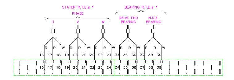
STATOR - 1 PER PHASE (3 LEAD TYPE)
