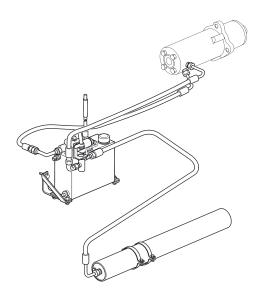
33.7 Hydralic starter unit mounted on right side 33.8 Hydralic starter unit mounted on left side 33.9 Hydralic starter, loose delivered
