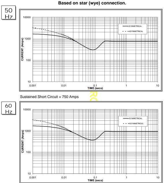
Three-phase Short Circuit Decrement Curve. No-load Excitation at Rated Speed Based on star (wye) connection.
