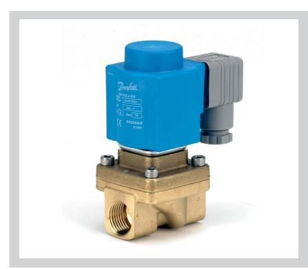
EV250B with assisted lift can operate from zero and up to 10 bar differential pressure. This 2/2-way valve program is especially to use in closed circuits with low differential pressure, but demanding moderate flow rates. Valve body in dezincification resistant brass for ensuring a long life even in connection with aggressive steam media.
